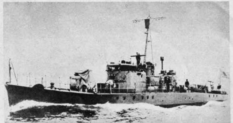
PC 40-44 Class subchaser has its stack set close to prominent bridge. A 33-knot ship, she is 146 ft. long and displaces 170 tons.
